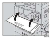
If the duplex unit is installed, close it by pushing up the catch.
